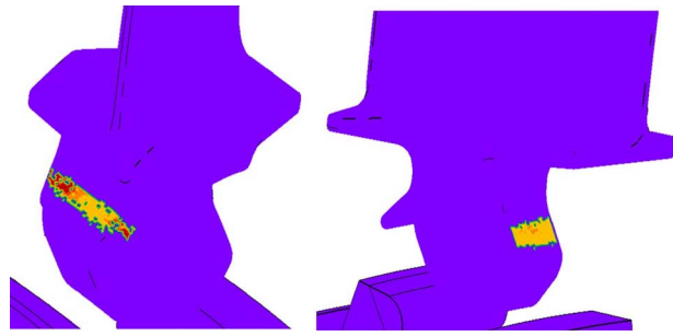
Fig. 15 Friction coefficient distribution on blade contact surfaces
